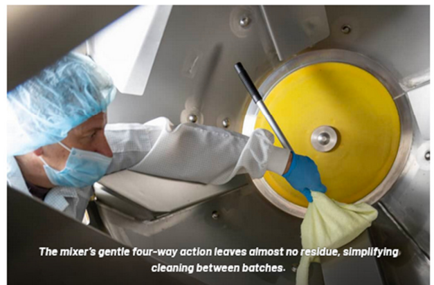
Internal mixing flights impart a tumble-turn-cut-fold action that produces a homogenous blend with no heat, shear or stratification.
