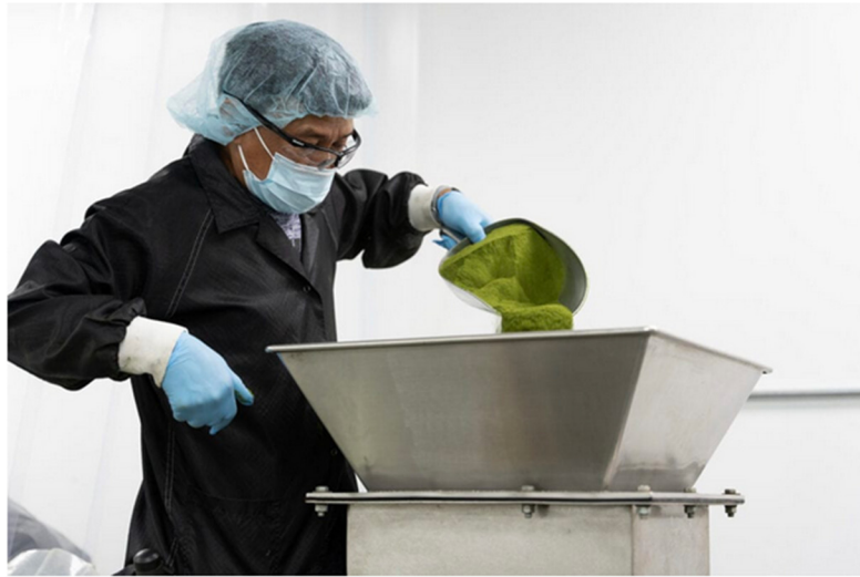
Operator empties a scoop of hand-weighed powder into the mixer intake which remains stationary as the vessel turns.
